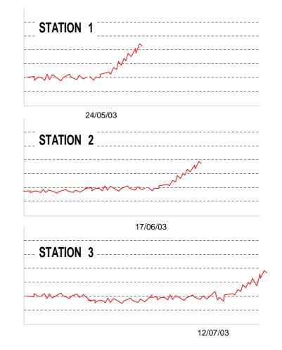
The station nearest the tree (Station 1) registered movement in late May. Station 2 followed less than a month later, and Station 3 registered movement on the 12<sup>th</sup> July. The roots of the Ash tree had changed the moisture content of the soil nearest to the tree first, and furthest away, last.
