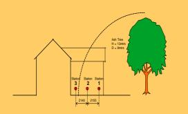
The Ash tree roots took approximately one month before influencing the moisture content of the soil sufficient to cause ground movement 2mtrs along the length of the wall between Stations 1 & 2.
