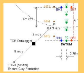
The Time Domain Reflectometry sensors propagate a high frequency transverse electromagnetic wave that is passed through four parallel 'prongs' buried in the soil. They measure the dialectric constant of the soil.
